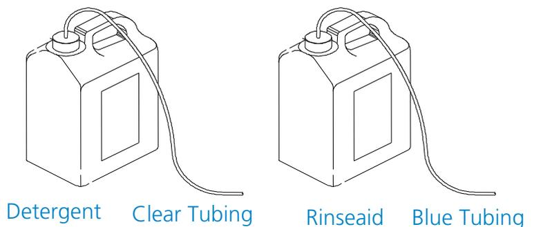
**Note:** Operating the machine without the correct chemicals or with chemical tubes wrongly connected to bottles will damage the ware and promote scale build-up.
