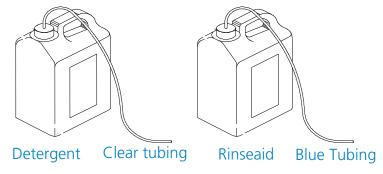
Note: Operating the machine without the correct chemicals, or with chemical tubes wrongly connected to bottles will damage the ware and promote scale build up.
